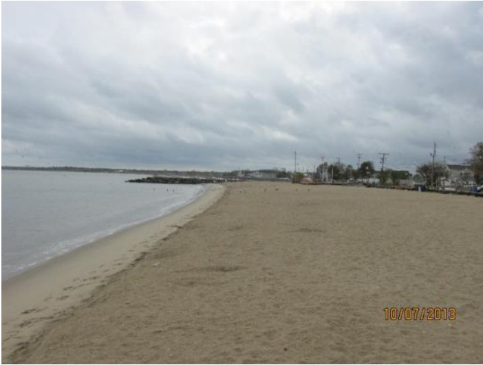
This site was moved to the public bathing beach in 2009. The photograph on the left shows the shoreline on October 7, 2013 following the addition of 14,000 cu. yds. of added sand. The photo on the right shows the adjustment in beach width over a year following the municipality’s efforts in replacing lost sand following Sandy (taken on October 7, 2014).
