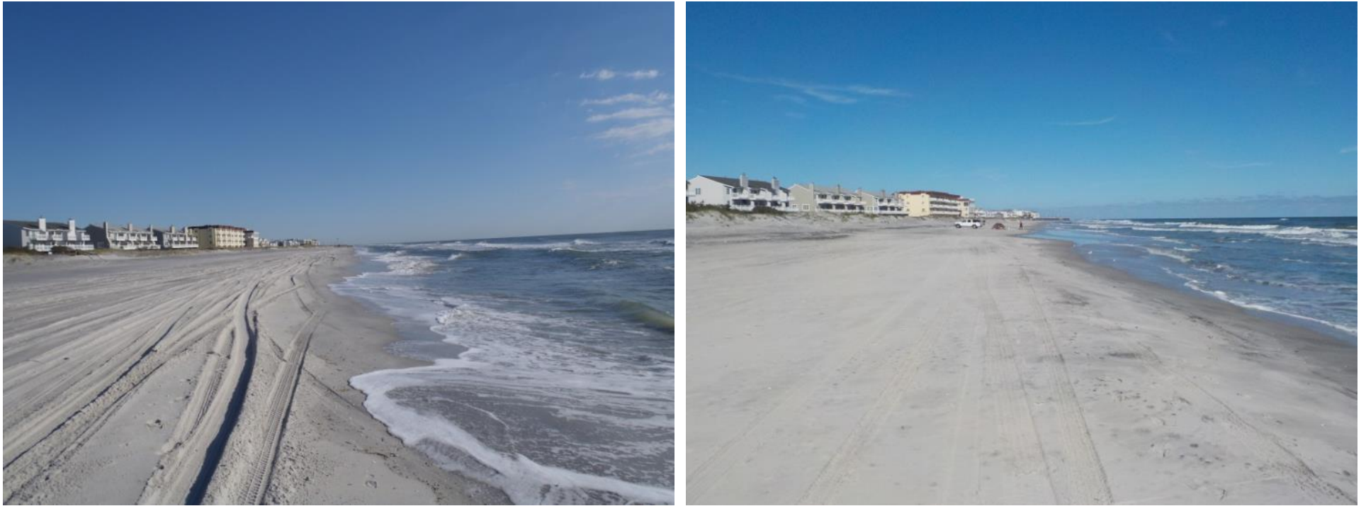
Figure 397a & 397b. This site is located within the engineered beach and federal project area. Positioned near the northern limit of development this site is just south of the erosional “hotspot”. Photo on the left was taken on October 16, 2015 shows a wide dry recreational beach. On the right (October 11, 2016), is the same view, one year later, shows little change in beach width or dune position.
