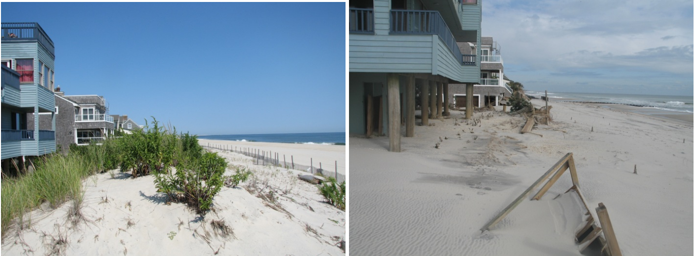
Above are two photos taken at La Baia Street before and after Hurricane Sandy. The photo on the left (taken September 12, 2012) shows the dune and beach conditions prior to the storm. In the photo on the right (taken November 2, 2012) the impact of the storm is evident. The former dune was removed and the shoreline moved 110.1 feet landward. Sand was overwashed between the oceanfront homes and carried landward to the road.
