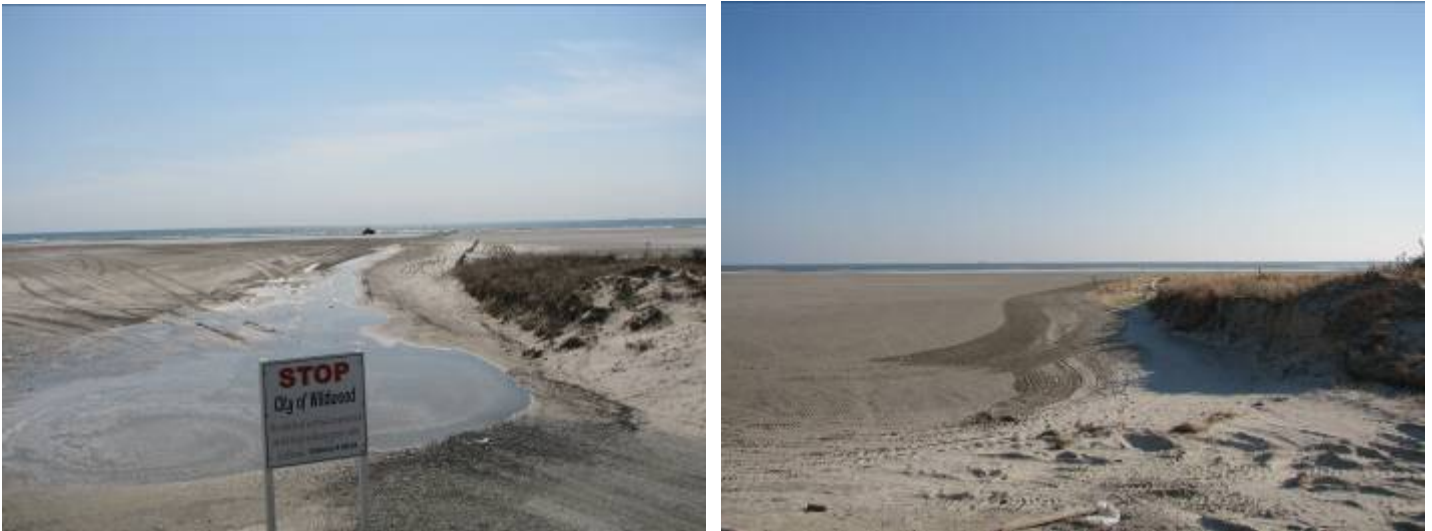
On April 4, 2012 the view across the beach in Wildwood was taken from the tiny dune in front of the boardwalk. The November 29 th view on the right was taken from the same location, but minus the sign. The beach gained sand at the berm 600 feet seaward of the boardwalk. The sand deposit probably was derived from the erosion of the spring survey's berm.
