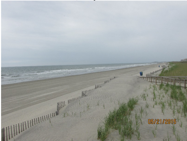
Photoplate 4a - Photo taken May 21, 2015. View to the south along the dune toe from 103 rd Street access pathway. The beach remained narrow from the previous fall survey. Wind-blown sand accumulated on the seaward dune slope that reduced the steep scarp and restored a gentler uniform slope.
