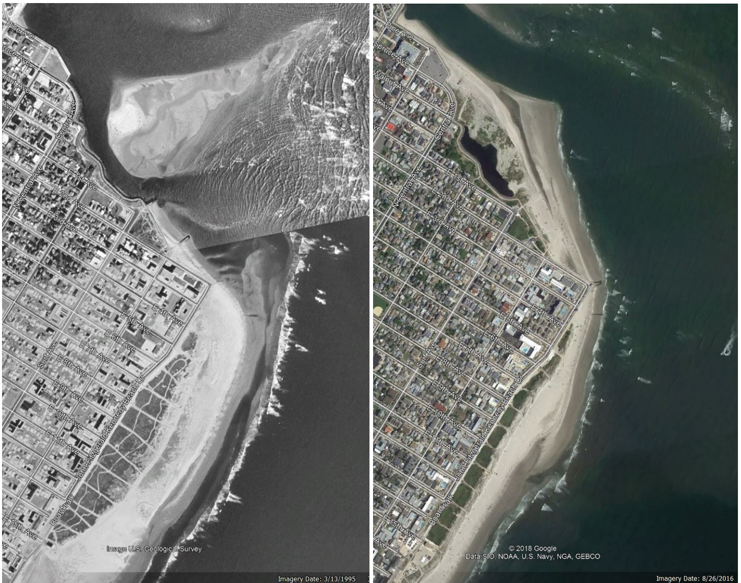
Figure 2. (Presented last year, but significant still). The northeast quadrant of the City of North Wildwood between March 1995 and August 2016 shows that oceanfront erosion appears related to large changes in shoal position and exposure at low tide in Hereford Inlet. In 1995, an exposed island sat between Central and Surf Avenues forcing a branch of the main tidal channel against the North Wildwood shoreline. There was no beach at the inlet shore until southeast of Surf Avenue. There was an extensive exposed sand flat system attached to the beach front bar system extending into the inlet. The ebb-tidal currents exited in proximity to the oceanfront beach and deposited sand in transport where wave action could easily move it to the beach bar system, and eventually onto the dry beach.
