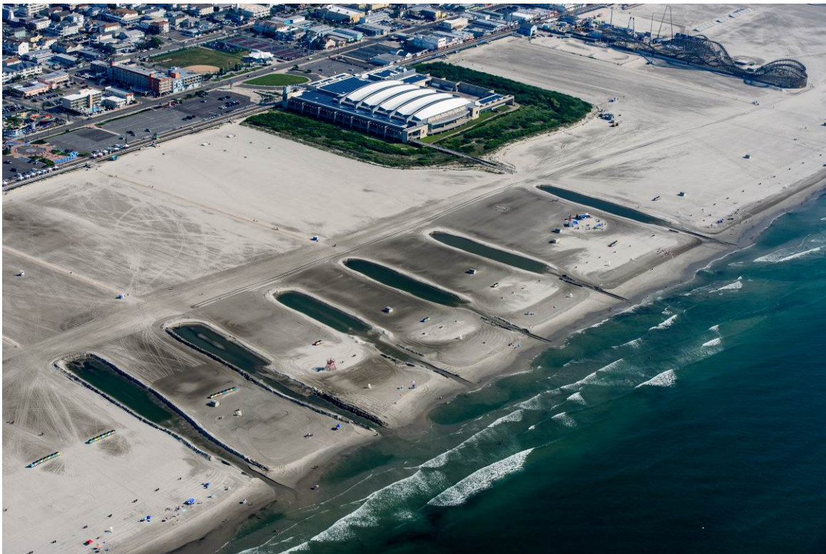
Figure 4. City of Wildwood oceanfront beach July 21, 2019 six weeks after conclusion of the 2019 back passing effort. The stormwater discharge points lie at the heads of each of the excavations at elevations well below the sand surface elevation. Burial means little effective stormwater discharge. They were originally built ending at the water's edge just past low tide. This view presents 20 – 25 years of evidence for shoreline accretion in the City of Wildwood.
